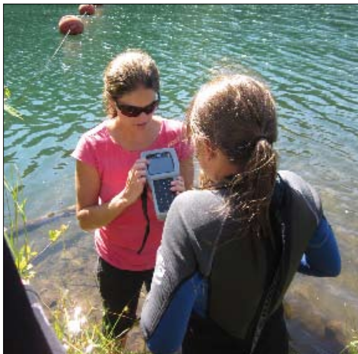
Columbia Riverkeeper's Water Quality Director, Lorri Epstein teaches a student how to use a YSI meter, which measures dissolved oxygen. Photo: Columbia Riverkeeper
