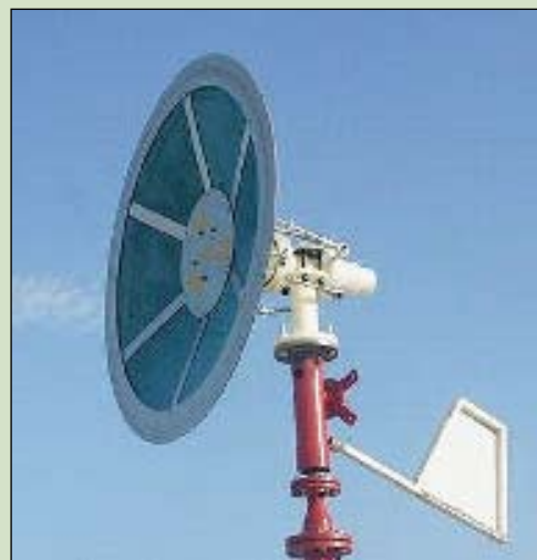
The new Saphonian wind turbine functions without blades. Photo: Saphon Energy
