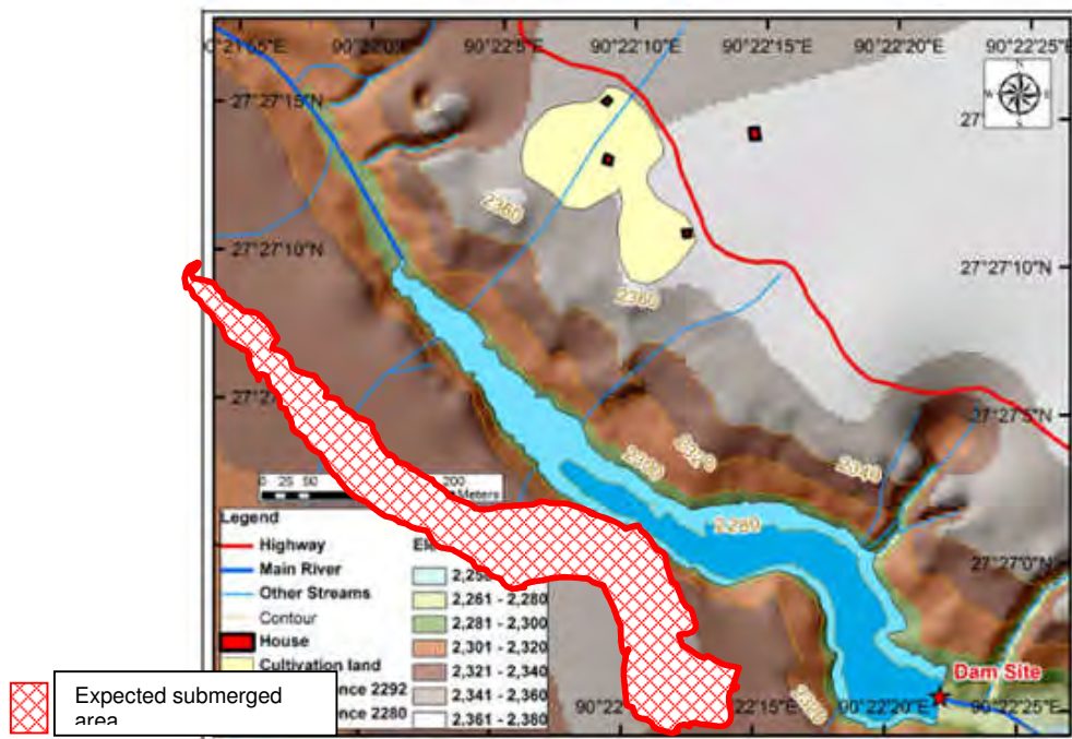
Figure 6-12: Expected submergence area above the diversion dam.
