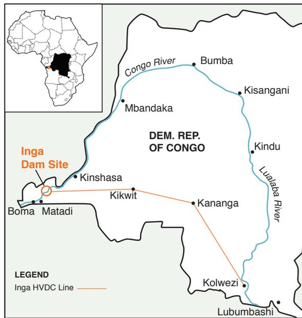
Budgeted at US\$250 million, actual construction costs quadrupled to \$1 billion. The Inga-Kolwezi high voltage direct current (HVDC) line was meant to deliver large amounts of electricity to copper mines in faraway Katanga Province, not cities or villages along its route. Within 10 years, poor maintenance, theft, and the ravages of the tropical climate caused the line to deliver less than half the electricity it was designed to carry.
